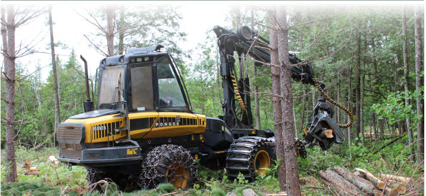
Photo: Cut-to-length harvester thinning a red pine stand on Lyme Great Lakes Timberlands property in Michigan
